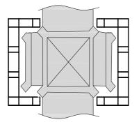
Fig. 4. Cross-section and location of scaffolding at ground level
